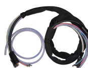
530360 (optional) 5 m, extension for wire feed unit with copper cable diam. 70 mm 2 ready for cooling unit.
